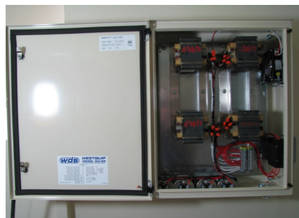
Weatherproof ballast box (CSA approved, individual breakers for lights, internal cooling fan, electrical cord with 30A 240V twistlock plug). Wall mount ballast box with quick change ballast and capacitor design for easy maintenance.
