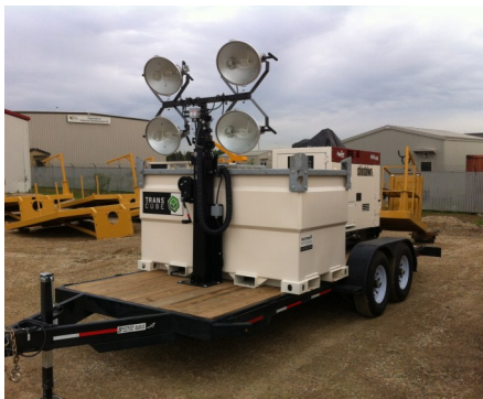
WQ5000S Light Mast System installed on open deck trailer with 2000L fuel tank and generator
